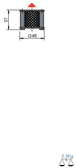
The triangles ▲ (shown on front view) and △ (shown on right-hand view) represent the assembled instrument. 2D or 3D drawings are available as an option to be specified in the order.
