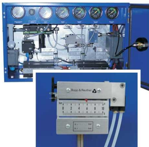
Upper picture shows pneumatic controller PC50 developed and manufactured for Bopp & Reuther Sicherheits- und Regelarmaturen GmbH, Mannheim with pneumatic precision pressure switches MANOCOMB® in special version (lower picture).
