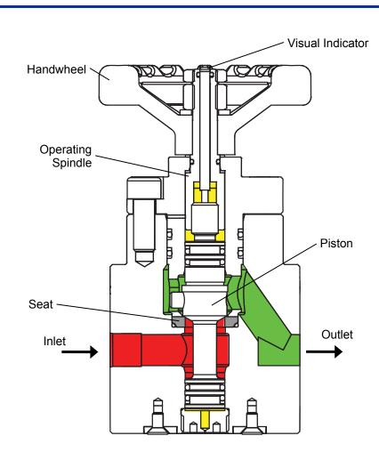
When the spindle is rotated by means of the handwheel, the piston moves vertically. The spindle has a left hand thread so the piston rises to open the valve when the handwheel is rotated clockwise. The piston is fully pressure balanced to minimise the load on the spindle.
